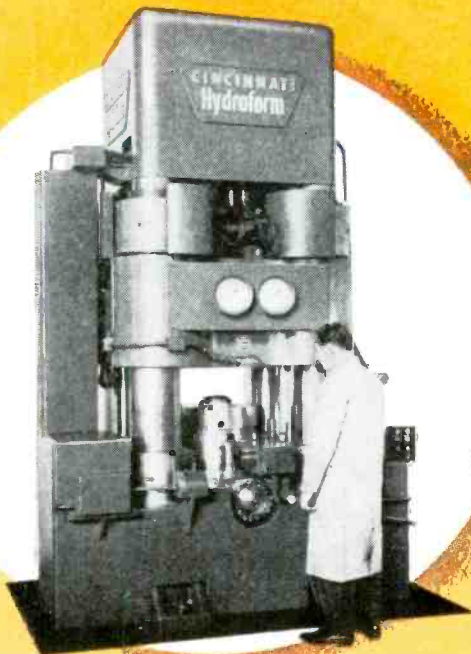
19-INCH HYDROFORM Maximum Blank 19" Diameter Maximum Draw Depth — 8"
