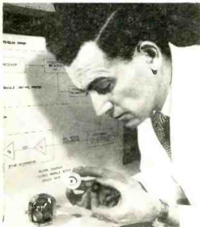
Doughnut of black, plastic-like solid propellant will be used to drive gyroscopic devices to be produced by Sperry Gyroscope. The gyroscope it drives, on table, can be accelerated up to speeds of 50,000 rpm in 0.2 seconds
