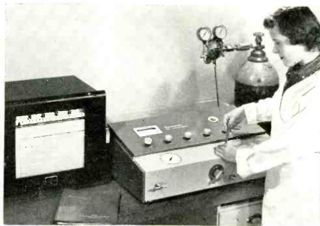
Operator uses syringe for injecting sample gas through rubber serum cap. Strip recorder is at left
