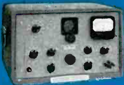
206A — very low distortion; for high quality, high accuracy audio tests. Covers 20 cps to 20 KC; output +15 dbm. $565.00.
