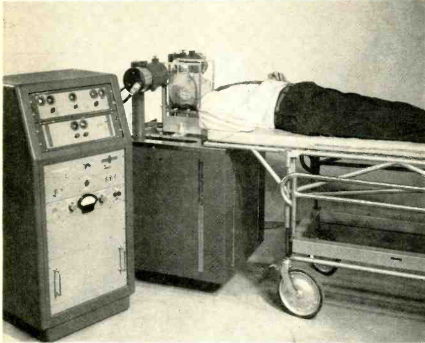
BRAIN TUMOR detector, that uses a radioactive arsenic source, is one of the new electronic devices shown at the Massachusetts General Hospital this month when three major groups gather in Boston to hear . . .
