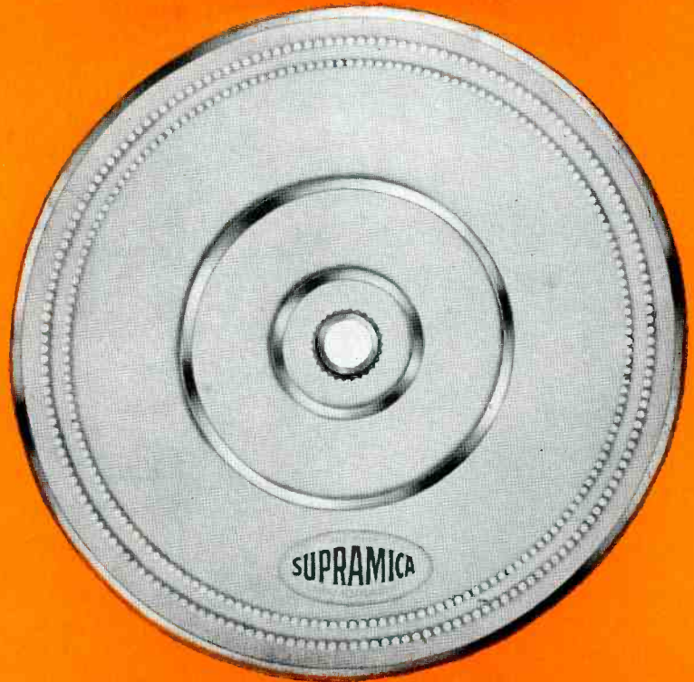
Precision-molded SUPRAMICA* 555 ceramoplastic Commutator Plate, CP-346, with 360 Contacts and 2 Slip Rings. Other Standard Plates are Available.
